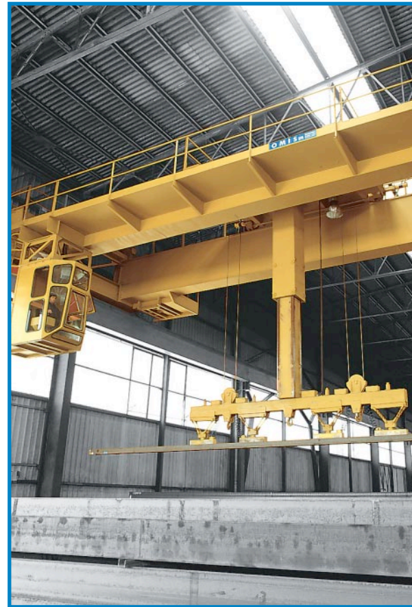
Bridge crane for handling steel beams, 2 winch trolleys with crossbeams (spreaders) and electromagnets, total carrying capacity 10 tonne, span 26 m.
