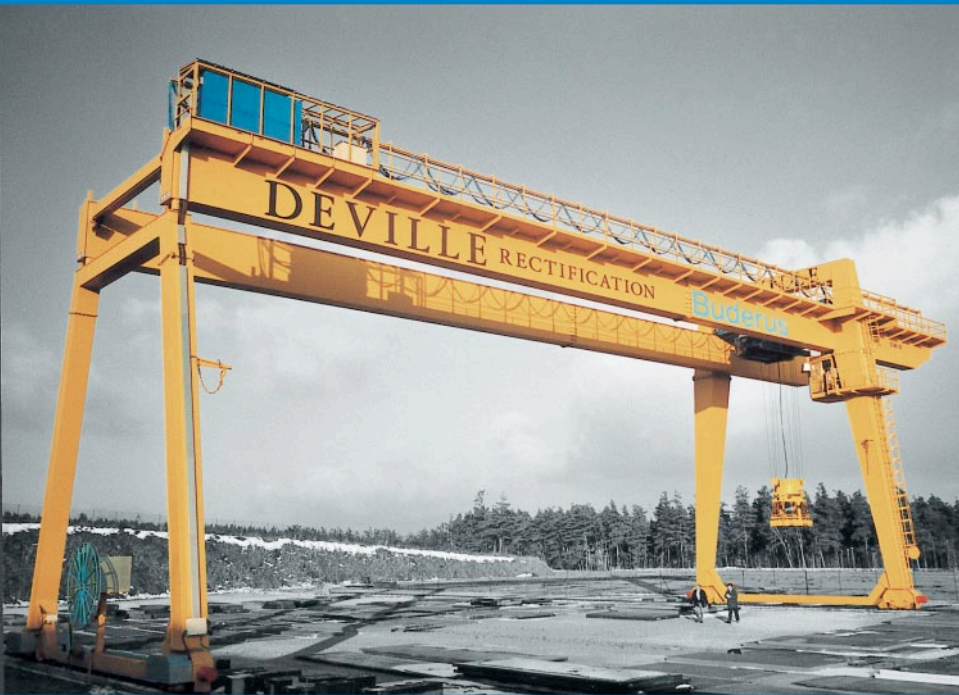
Gantry Crane for an iron deposit, 25 tonne capacity (12,5 + 12,5), span 35 m + 10 m of jut, height 17 m, trolley with a double 360° rotating winch. Bridge speed 60 m / min with frequency control.
