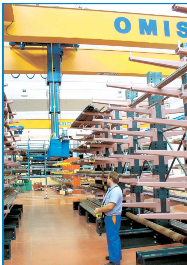
Double girders bridge crane with load charging system guided through telescopic guides.
