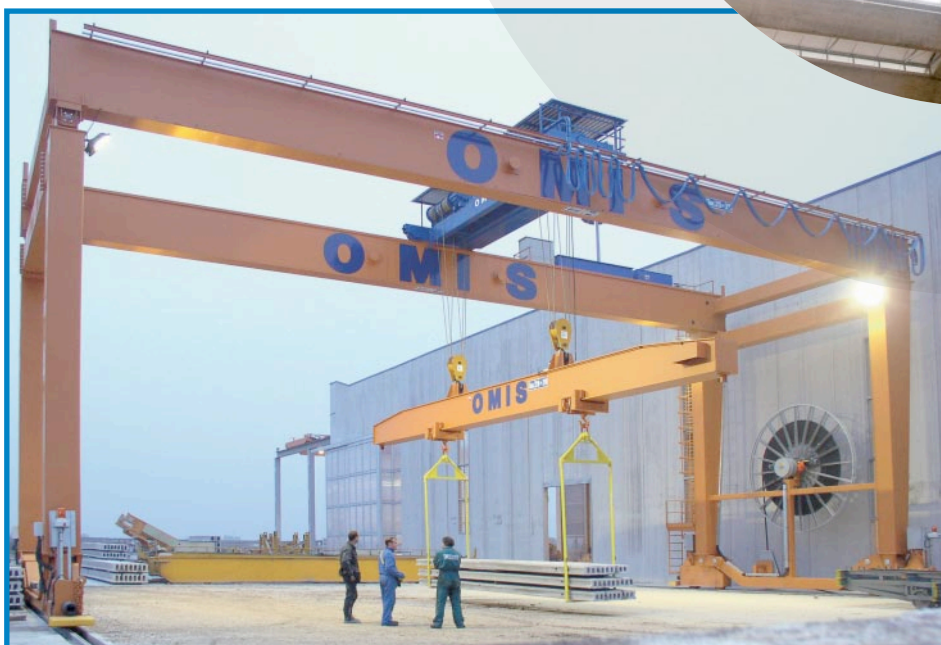
Double girder bridge crane capacity 6,3+6,3 with two independent hoist trolleys. Traversers (transfer tables) for zincing / galvanising plants.
