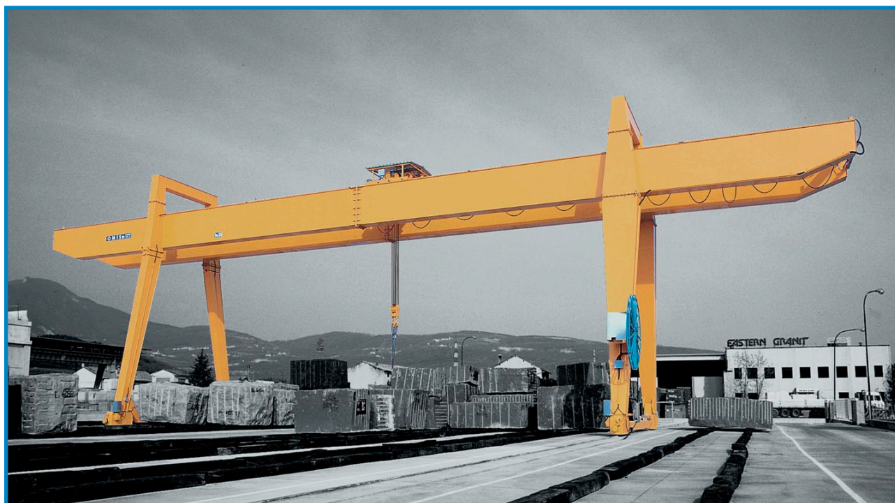
Stone and marble yard gantry crane, 35 tonne span 25 m and 8,5 m of jut on each side
