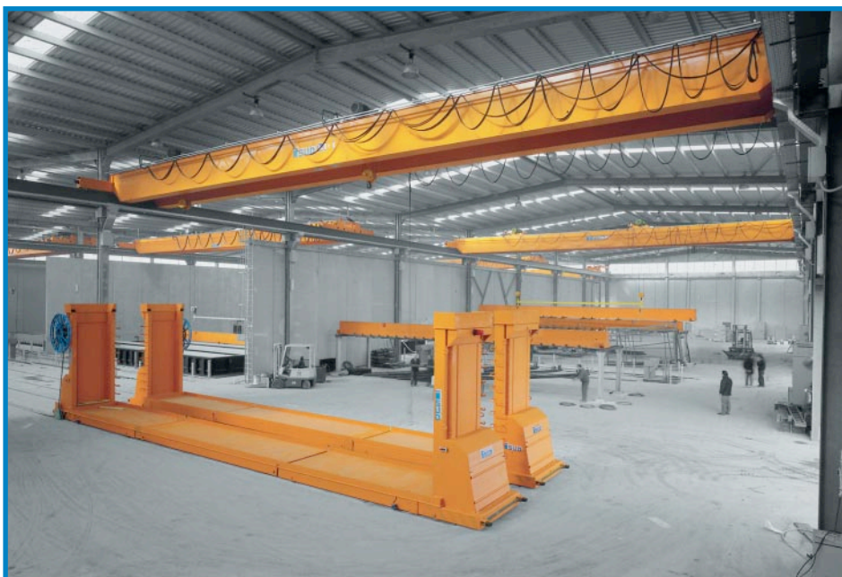
Double girder bridge crane capacity 6,3+6,3 with two independent hoist trolleys. Traversers (transfer tables) for zincing / galvanising plants.
